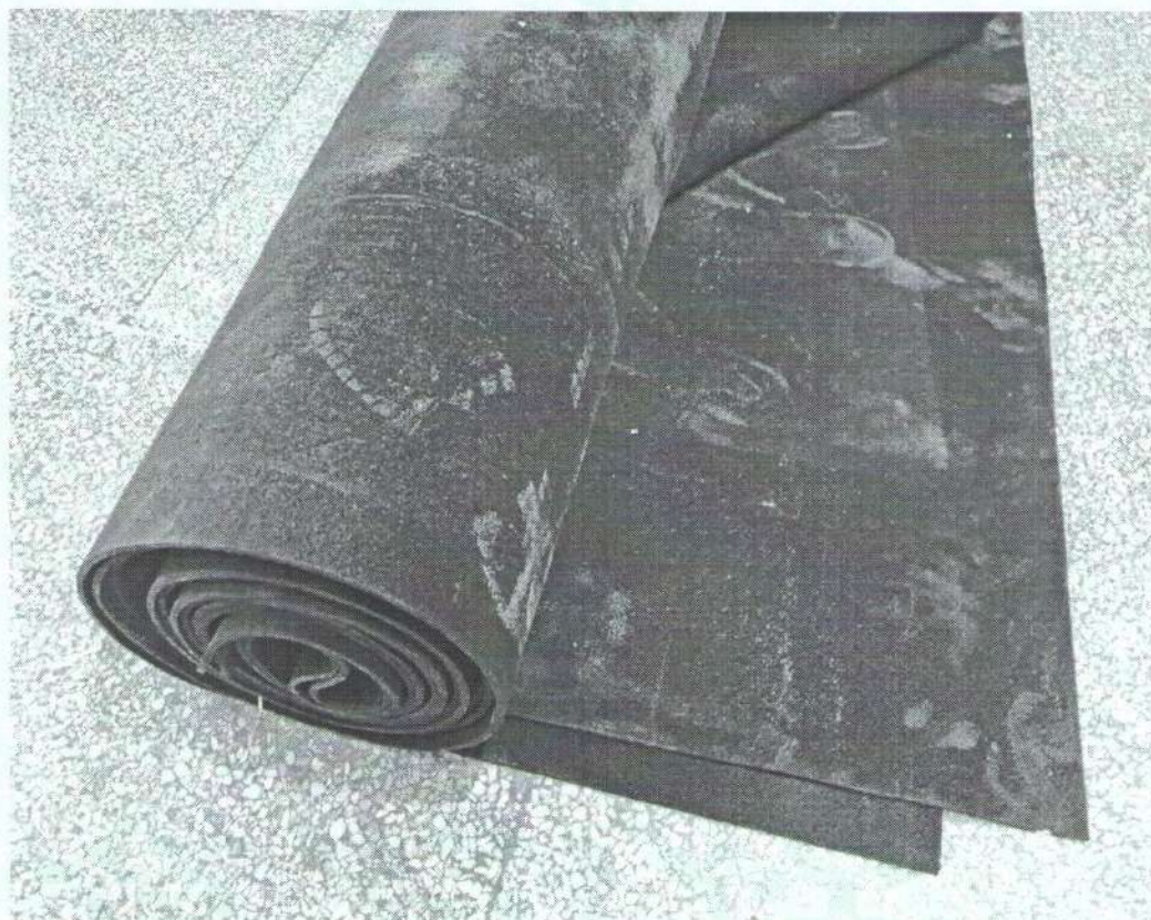
5mm 减震隔声垫 5mm Acoustic Underlay
